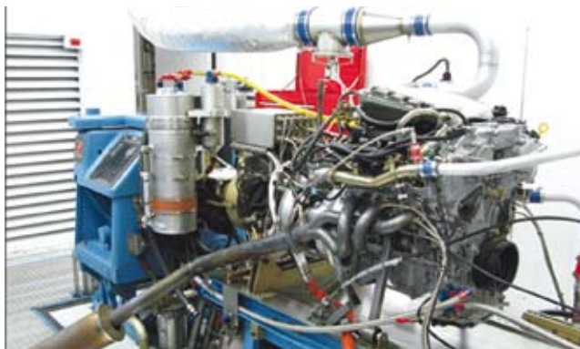
Engine rig-up in a dynamometer (source: http://www.modified.com/ )
